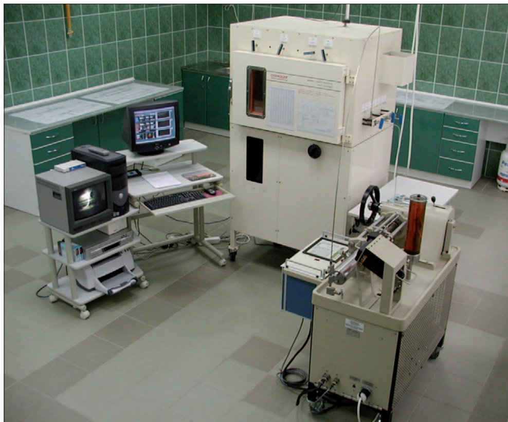
Rys. 3.2. Aparatura do badań PVT firmy Chandler Engineering – Model 2370-3000-G PVT System [81]
