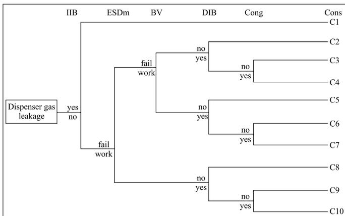
**Figure 3.** The event tree of the dispenser gas leakage
