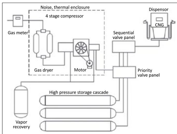
Figure 1. Components of a CNG station (Chinese et al., 2014)
