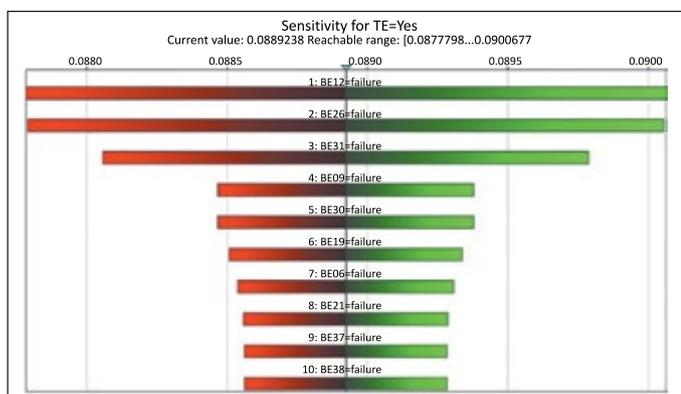
**Figure 6.** Tornado Diagram showing the top 10 critical basic events for dispenser gas leakage
