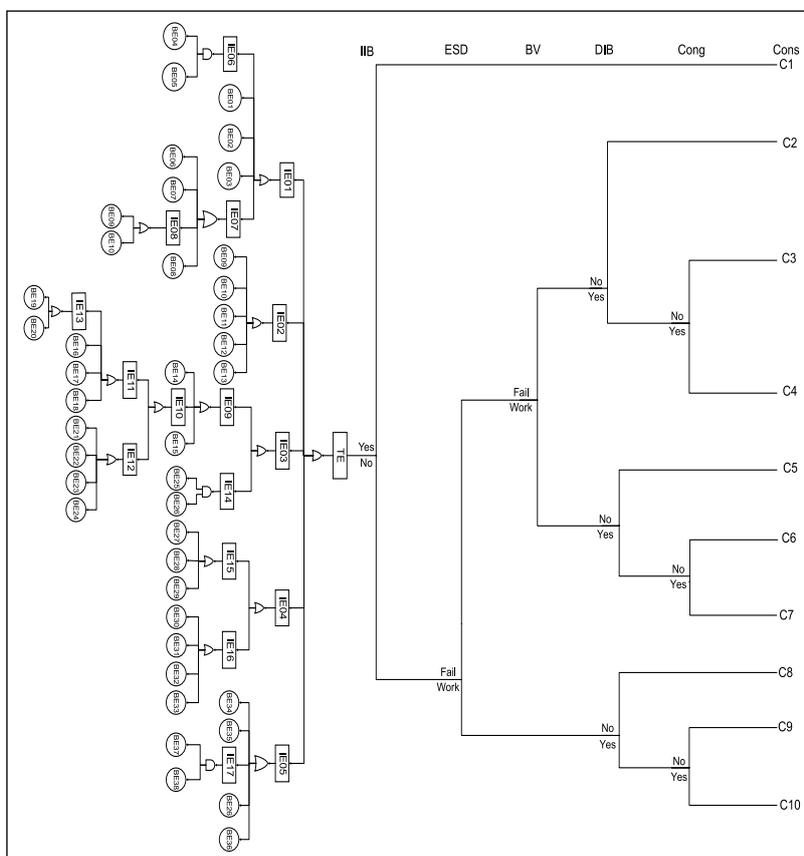
**Figure 4.** Accident scenario modeling of the dispenser gas leakage using Bow-tie approach
