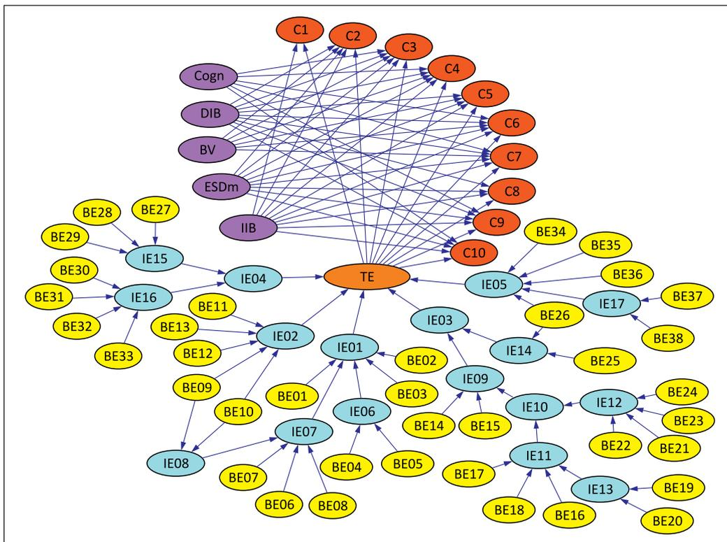
Figure 5. Dynamic cause-consequence analysis of the dispenser gas leakage using BN
