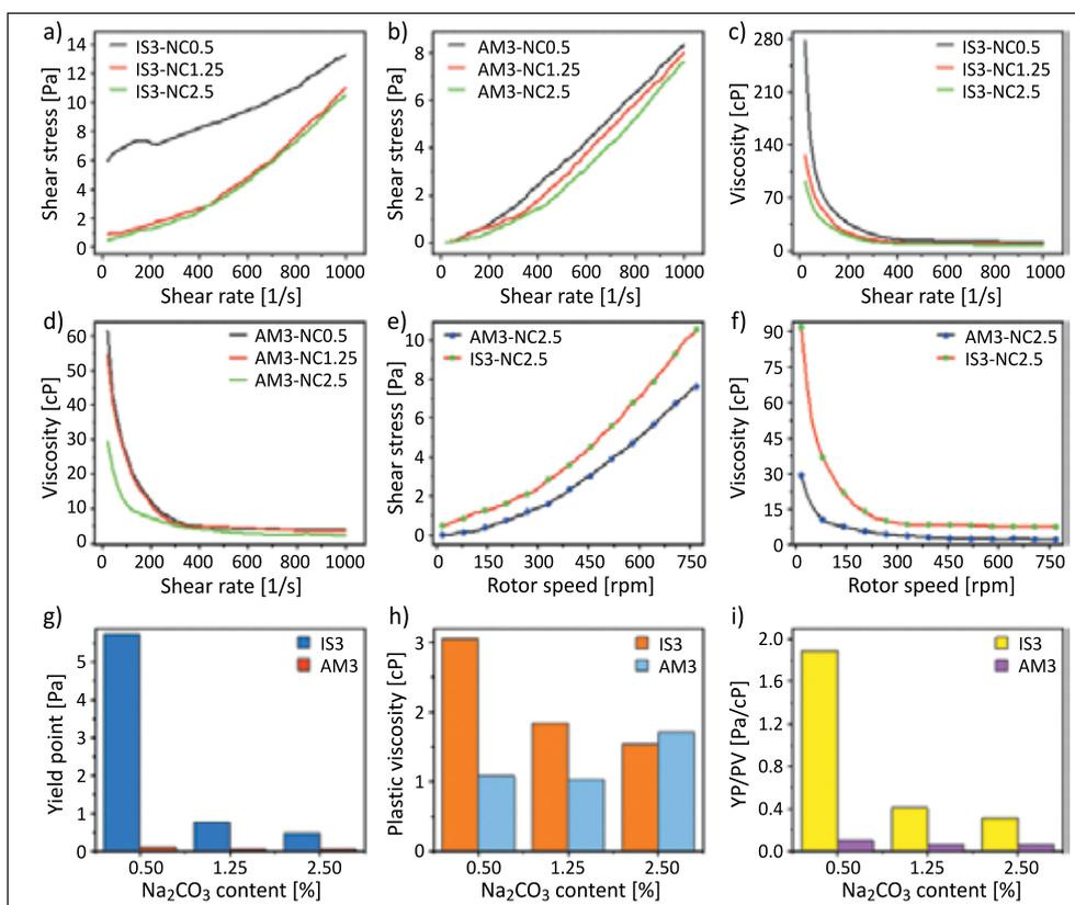
**Figure 7.** Shear stress and viscosity versus shear rate for  $\text{Na}_2\text{CO}_3$  modified IS3 and AM3 bentonites (a–d); yield point variation with  $\text{Na}_2\text{CO}_3$  (e); comparison of shear stress and viscosity for the high  $\text{Na}_2\text{CO}_3$  content (2.5g) modified clays (f–g); plastic viscosity and YP/PV variation with  $\text{Na}_2\text{CO}_3$  content (h–i)
