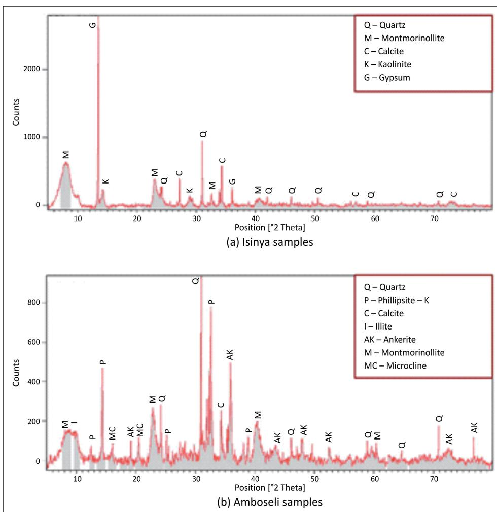
**Figure 6.** Mineralogical analysis of Isinya (a) and Amboseli (b) bentonite samples
