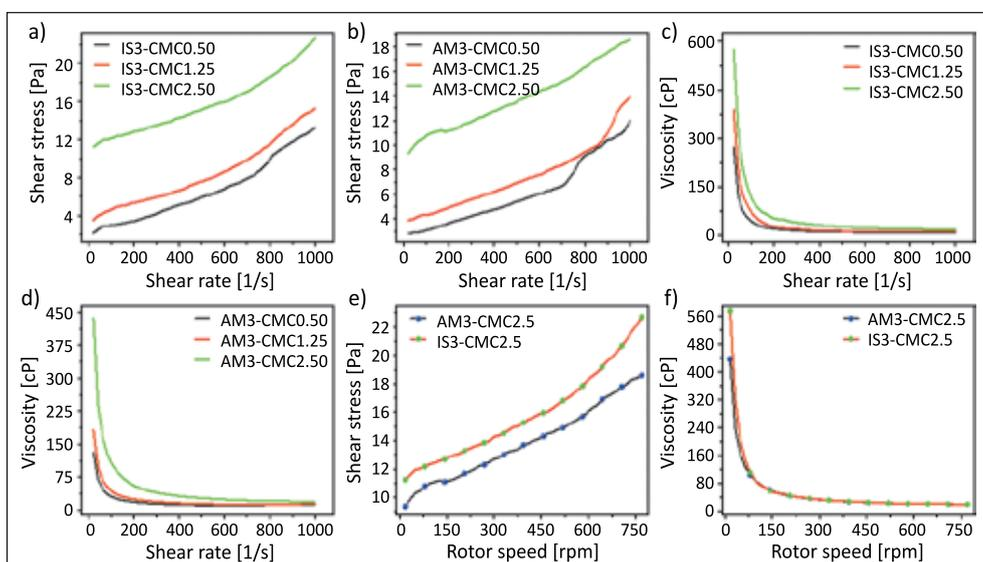
**Figure 8.** Shear stress and viscosity versus shear rate (a–d), and comparison of shear stress and viscosity against rotor speed (e–f) for the CMC-modified bentonites
