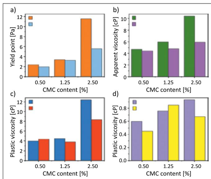
**Figure 9.** Yield point, apparent viscosity, plastic viscosity, and YP/PV versus CMC content for IS3 and AM3, respectively
