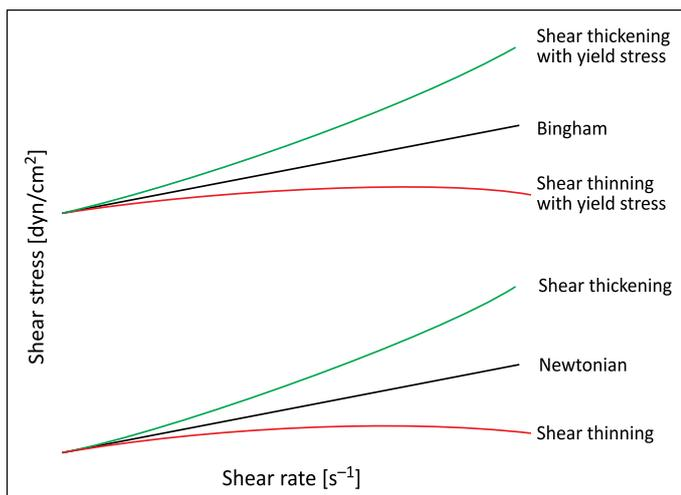
**Figure 3.** Rheological properties of both Newtonian and non-Newtonian fluids (according to Jankowska et al., 2023)
