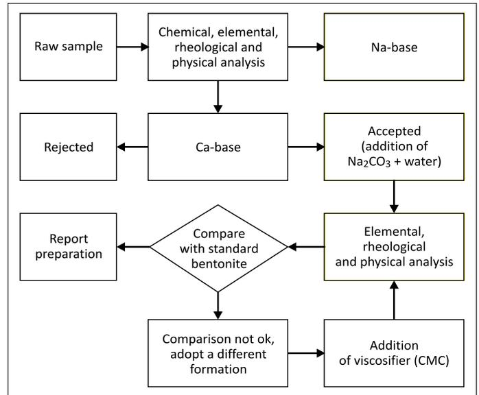
Figure 2. Flowchart illustrating the beneficiation procedure of the raw bentonite with either sodium carbonate or carboxymethyl cellulose (CMC)
