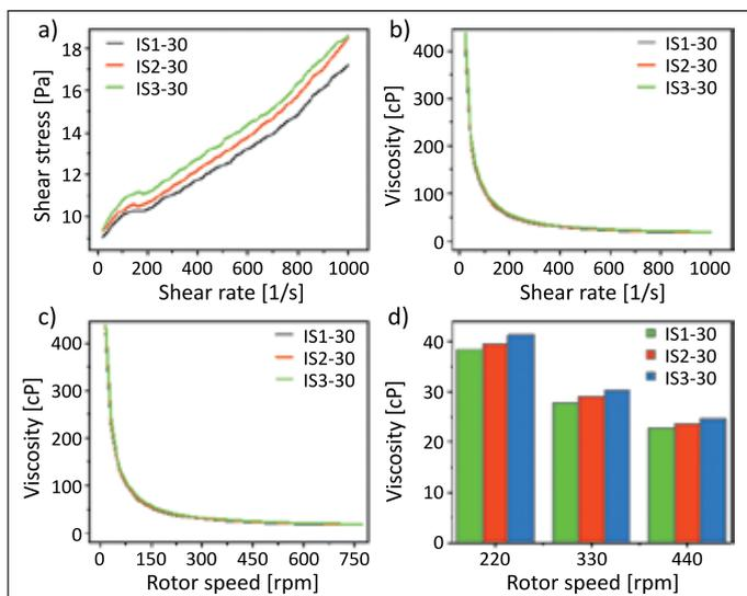
**Figure 5.** Variation in shear stress (a) and viscosity (b) versus shear stress, and viscosity of 30w% versus the rotor speed (c–d) for IS1-3 suspensions
