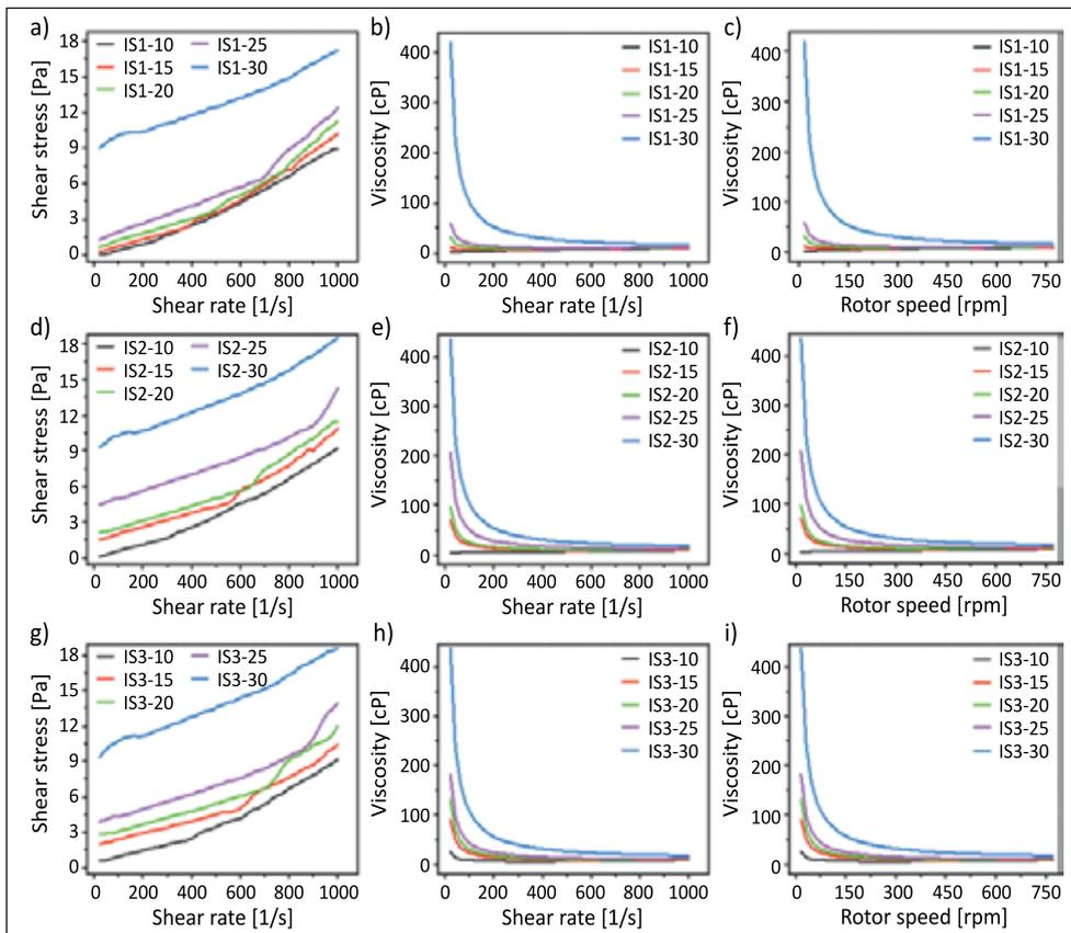
Figure 4. Shear stress versus shear rate (a–c); viscosity versus shear rate (d–f); and viscosity versus the rotor speed (g–i) for IS1-3 samples
