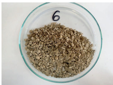
Fig. 12. Miocene shale recovery after dispersion at 80°C in drilling mud, the drilling mud containing 3% R2100 and 1% emulsifier (drilling mud 7, tab. 3)
