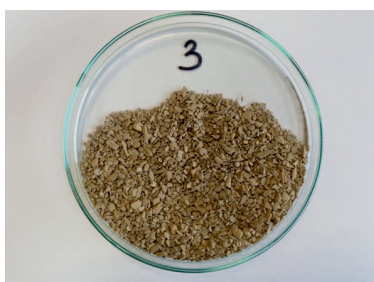
Fig. 15. Miocene shale recovery after dispersion at 80°C in water, the drilling mud containing 3% OL2024 and 1% emulsifier (drilling mud 9, tab. 3)
