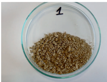
Fig. 11. Miocene shale recovery after dispersion at 80°C in water the drilling mud containing 4% P600 (drilling mud 5, tab. 3)
