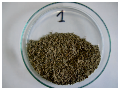
Fig. 7. Miocene shale recovery after dispersion in water at 80°C after previous dispersion in drilling mud containing 4% OL200 (drilling mud 3, tab. 3)
