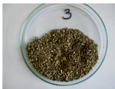
Fig. 9. Miocene shale recovery after dispersion at 80°C in water after previous dispersion in drilling mud containing 4% OL2024 (drilling mud 4, tab. 3)
