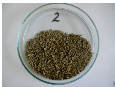
Fig. 5. Miocene shale recovery after dispersion in water at 80°C after earlier dispersion in drilling mud containing 4% OL700 (drilling mud 2, tab. 3)
