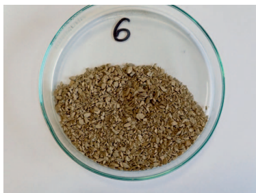
Fig. 13. Miocene shale recover after dispersion at 80°C in water after previous dispersion in drilling mud containing 3% R2100 and 1 % emulsifier (drilling mud 7, tab. 3)
