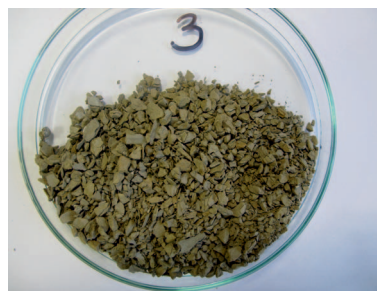
Fig. 8. Miocene shale recovery after dispersion in drilling mud at 80°C the drilling mud containing 4% OL2024 (drilling mud 4, tab. 3)
