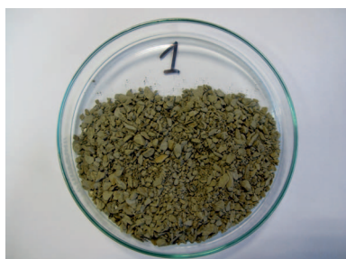
Fig. 6. Miocene shale recovery after dispersion in drilling mud at 80 °C, mud containing 4% OL200 (drilling mud 3, tab. 3)
