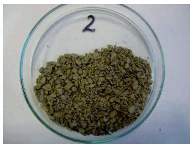
Fig. 4. Miocene shale recovery after dispersion at 80 °C in drilling mud containing 4% OL700 (drilling mud 2, tab. 3)
