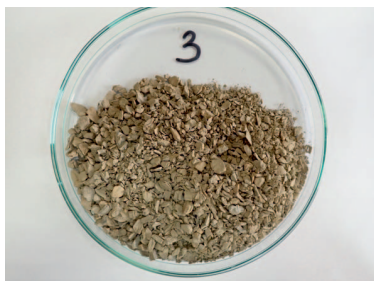
Fig. 14. Miocene shale recovery after dispersion at 80°C in drilling mud, the drilling mud containing 3% OL2024 and 1% emulsifier (drilling mud 9, tab. 3)
