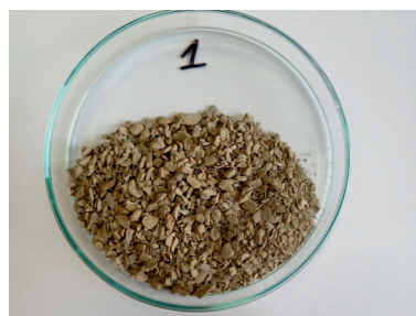
Fig. 10. Miocene shale recovery after dispersion in drilling mud at 80 C the drilling mud containing 4% P600 (drilling mud 5, tab. 3)
