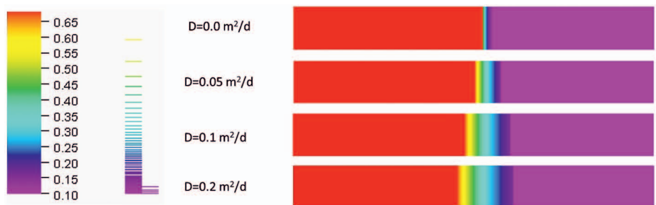
Fig. 7. The effect of taking into account physical dispersion. Water saturation in the model blocks
