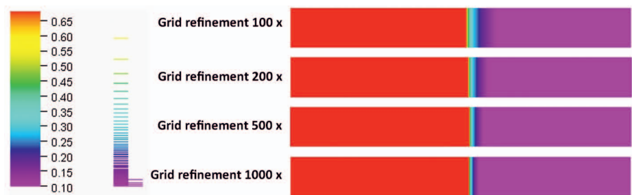
Fig. 6. Numerical dispersion limitation. The effect of using a double discretization grid with triple weighing during fluid mobility calculations. Water saturation in the model blocks
