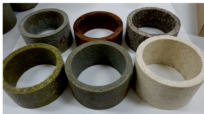
Fig. 2. Fuel samples extruded in a ring-shaped form and prepared for shooting tests: (a) Sz/KClO 4 /PAM propellant granules; (b) Sz/Szd/KClO 4 /PAM propellant granules; (c) R/KClO 4 /PAM tube propellant granules; (d) Coiled M-type propellant ring – manufactured by ZPS Gamrat Jasło; (e) R-type tube propellant granules
