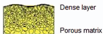
Fig. 1. A section through the UBE polyimide membrane tested as part of laboratory tests [34]
