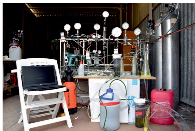
Fig. 5. Photos of the membrane gas separation test stand
