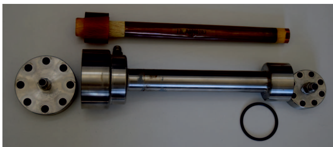
Fig. 3. A photo of a hollow-fibre membrane bundle and a module housing for membrane separation
