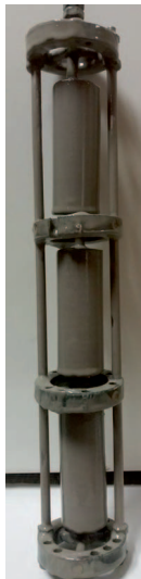
Photo 5. Cores with a filter cake (after washing with drilling mud)
