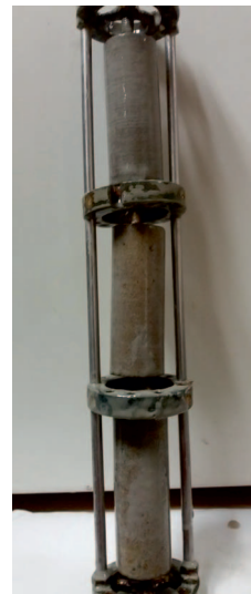
Photo 8. Contact time 8 min at the pumping rate of 11.2 [l/min]
