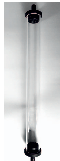
Photo 4. View of the plastic pipe together with sealants, in which the drilling fluid inlet and outlet have been fixed
