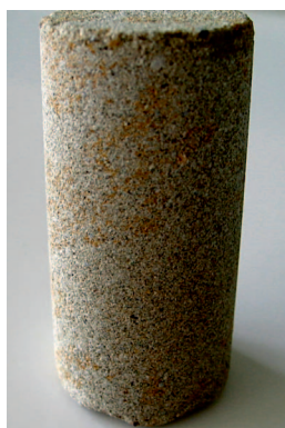
Photo 2. Core cut out of a sandstone specimen
