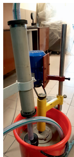
Photo 1. Borehole drilling fluid flow simulator (the device is in the course of pumping fluids)
