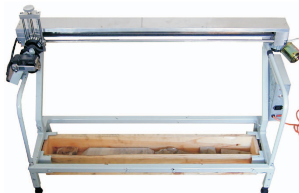
Fig. 2. The portable unit for drill core photography
