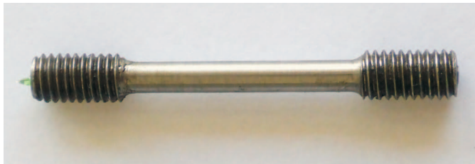
Photo 3. Example of a specimen before SCC testing
