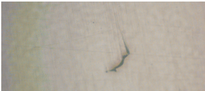
Photo 8. Crack #1 observed on specimen 2C of L360NB steel at 100x magnification
