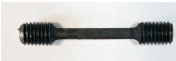
Photo 5. Example of specimen that passed SCC test
