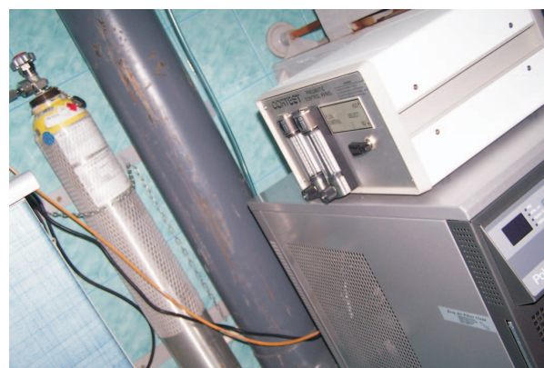
Photo 7. Equipment for maintaining HIC test conditions in the test chamber
