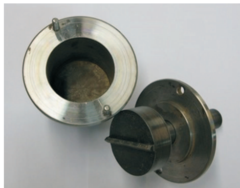
Fig. 2. Mortar used to crush samples so as to eliminate the loss of mass
